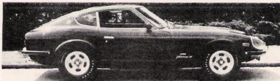
OSTENSIBLY a stock Z-car, this 432 gets a subtle badge, wide mags, fat boots, and headlight fairings for identification. Nit-picking regulations eliminate the headlight fairings in Australia.
